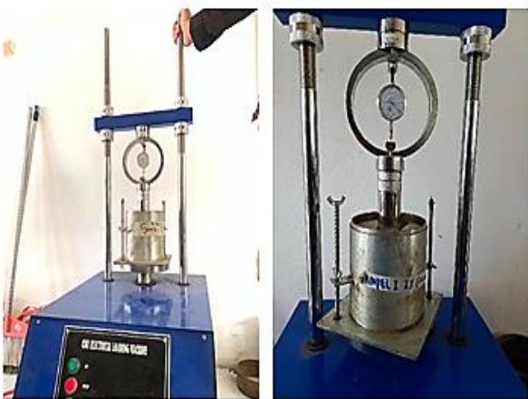
Figure 3: CBR Testing Process
