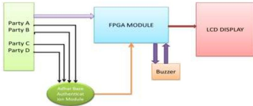
Fig 1. Block diagram of EVM
