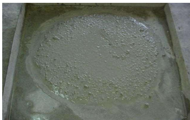
Figure 20: Results of slump flow Test
