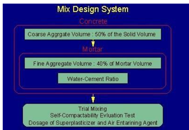
Figure 6: Schematic diagram showing mix design system.
