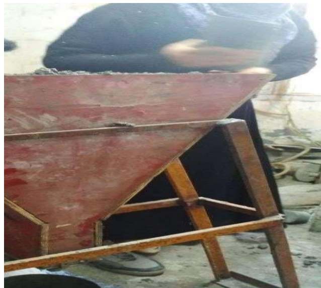
Figure 21: Locally fabricated V-Funnel utilized to evaluate the segregation resistance of SCC
