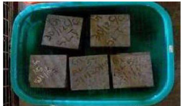
Figure 3: Sample dipped in Diluted 5 % Sodium Sulphate Solution
