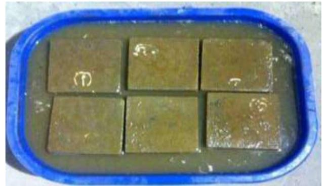
Figure 2: Sample submerged in 3% diluted sodium chloride solution
