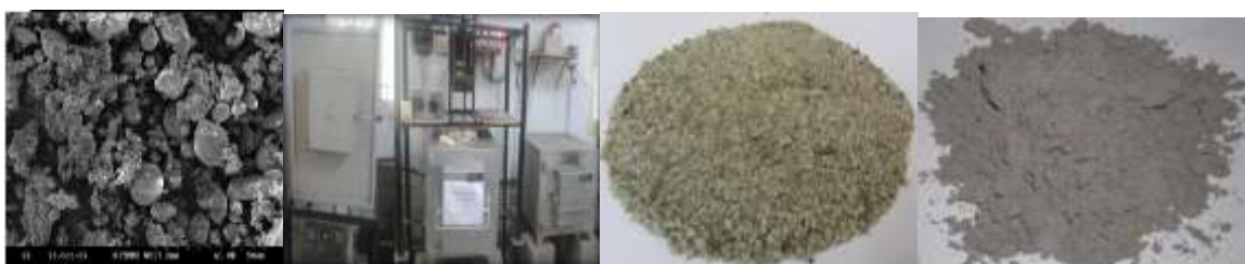
Figures 1: a) SEM micrographs of fly ash particles SEM of AA 2024 alloy -% fly ash b) Stir Casting Set-up used for fabrication of Composites and the fly ash powder of pre heat condition GBF) slag powder and fly ash
