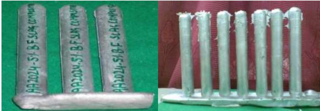
Figure 2: As cast cylindrical fingers of Al based metal matrix composite (a) Al-5% wt. GBF) slag reinforced composite (b) Al- 5% wt. fly ash reinforced (ALFA) composite
