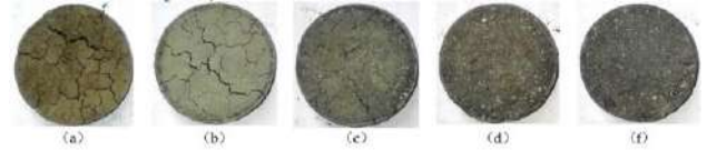
Figure 6: Crack morphology of ES with RHA-CCR content (curing time = 28 days) (Liu et al., 2019).
