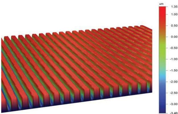
Figure 4: Optical profiler measurement performed on a B type coil after the seed layer deposition
