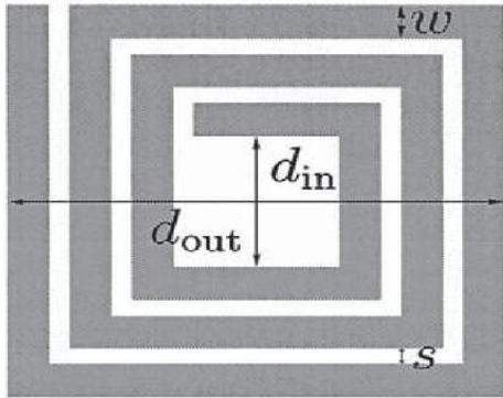
Figure 1: Parameters for the computation of the Wheeler's formula [1].
