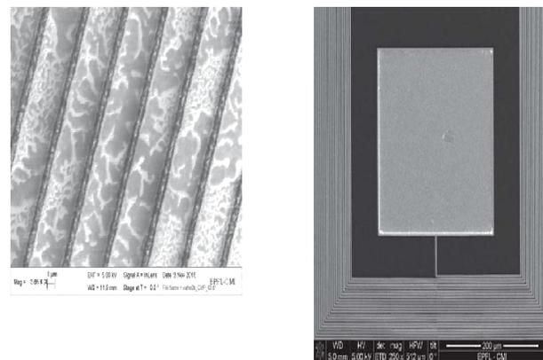
Figure 5: Surface contamination by slurry silica particles after CMP
