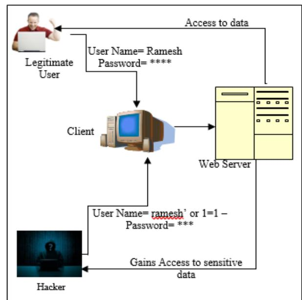
Figure 1: SQL Injection Attack Working
