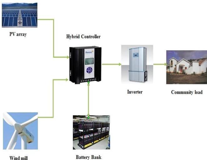
Figure 2: PV-wind hybrid system
