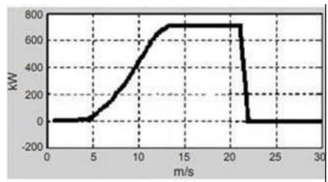
Figure 1: A typical machine power curve in a wind tunnel
