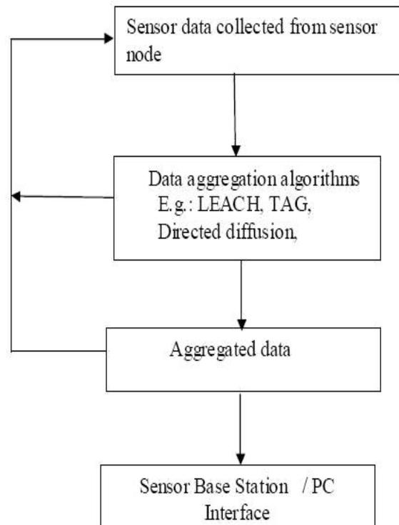
Figure 3: General architecture of the data aggregation algorithm
