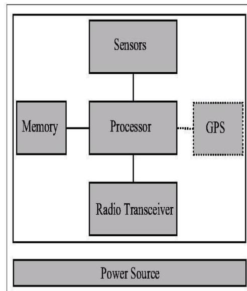
Figure 1: Basic Components of a WSN Node
