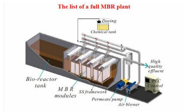
Figure 1: Treatment of Wastewater using Membrane Bioreactors [YX-FILTER]
