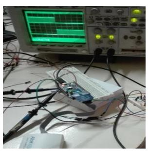
Figure 4: Test setup with ARM ULINKpro-D
