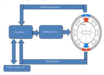
Figure 1: Block diagram for Embedded Ceiling Fan
