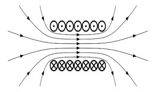
Figure 2: Magnetic field produced by a solenoid (coil of wire)
