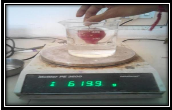
Figure 3: Shows the Measurement of volume, true density, and specific gravity of Cactus Pear.
