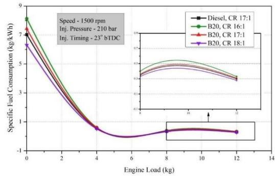
Figure 5: Specific fuel consumptions Vs load at different compression ratios
