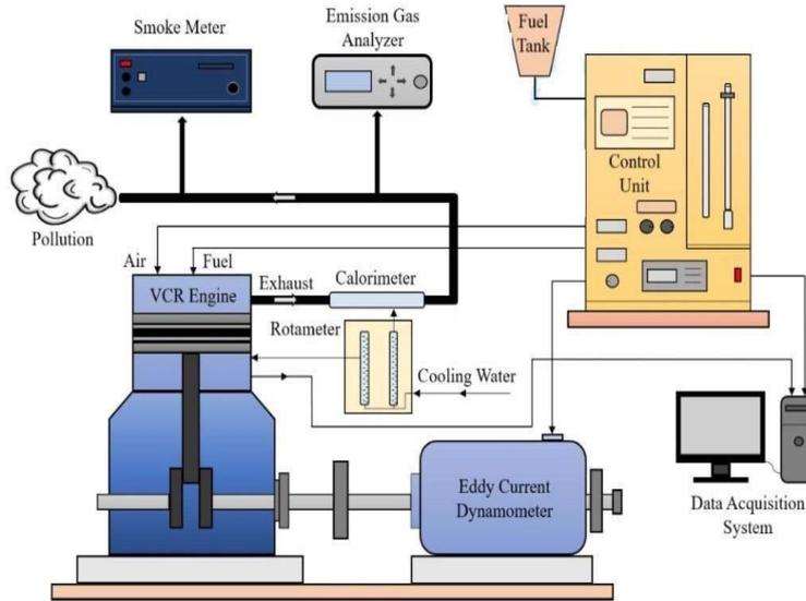
Figure 1: Schematic Representation of Engine Layout
