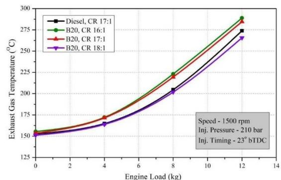
Figure 6: Exhaust gas temperature Vs load at different compression ratios
