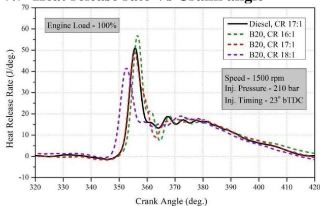
Figure 11: Heat release rate Vs Crank angle at different compression ratios
