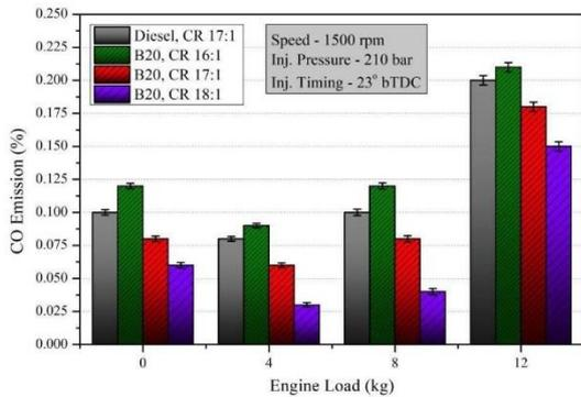
Figure 7: CO emissions Vs load at different compression ratios
