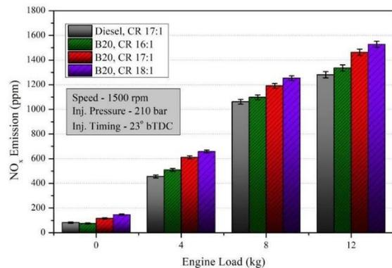
Figure 9: NO<sub>x</sub> emissions Vs load at different compression ratios
