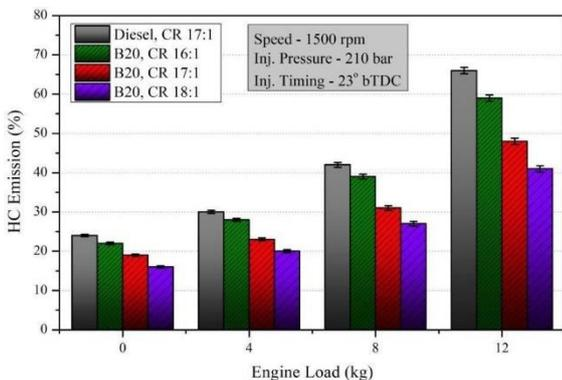
Figure 8: HC emissions Vs load at different compression ratios
