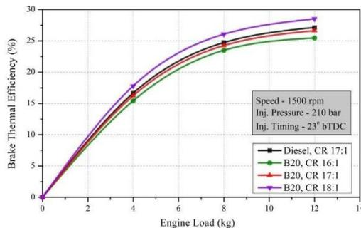
Figure 4: Brake Thermal Efficiency Vs Load at Different Compression Ratios
