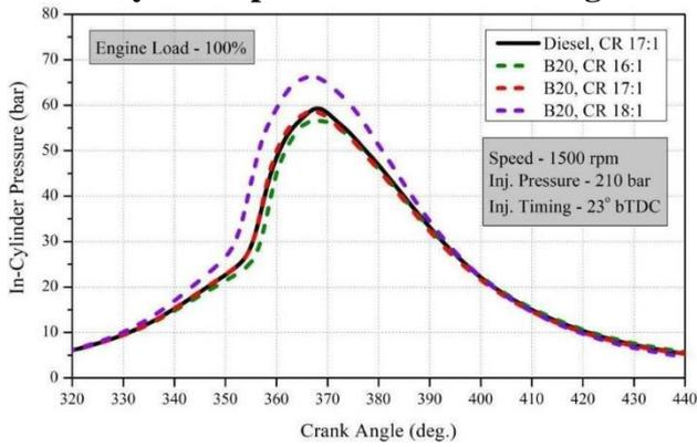
Figure 10: In-cylinder pressure Vs Crank angle at different compression ratios
