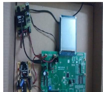
Fig. 1.1 RFID BASED SHOPPING CART
