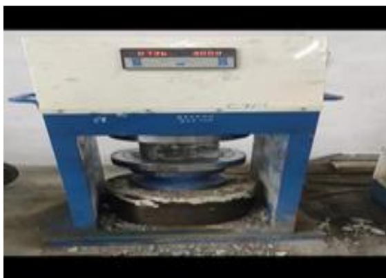
Figure 2: Compression testing machine with maximum capacity of 3000 Kn
