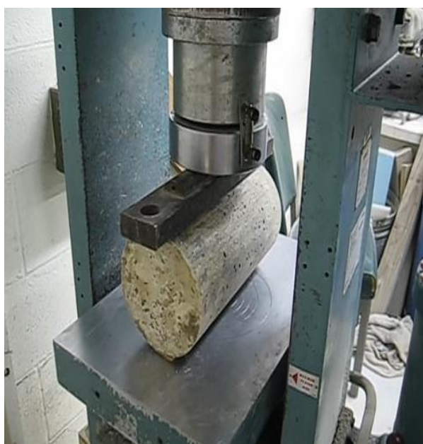
Figure 2: split strength testing apparatus
