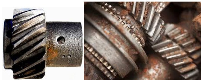
Fig.5. Brown coloration of materials due to corrosion
