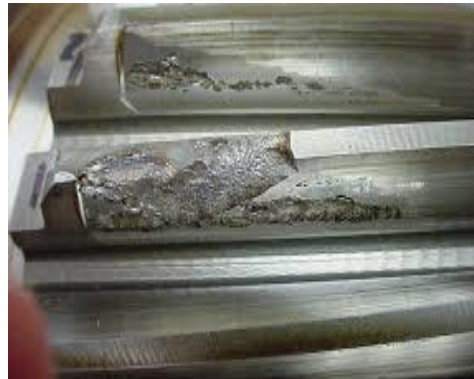
Fig.1. Spalling of helical gear teeth
