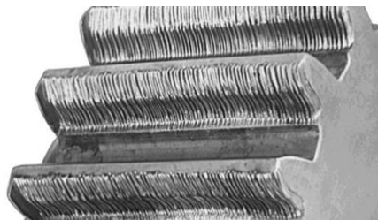
Fig.4. Fine lines over material due to abrasive particles
