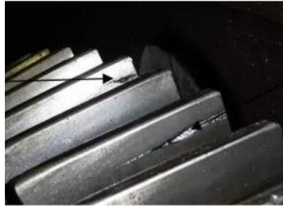
Fig.3. Teeth cracks near gear root due to low bending stress of material
